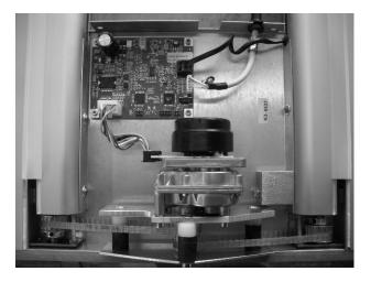
Exchange the defect printed circuit board. Put in the cables at the same position. (Pay attention to the code) Rebuild the casing. Perform a reference run. See chapter 7.4 Finally, a function- and safetytest has to be performed.
