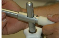
8) Adjust femoral and tibial plates for right or left leg by loosening white knob.
