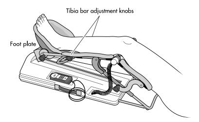
**9.** Wrap the Pad Strap around the thigh, femur bars and pad to secure the patient's leg to the FLEX-MATE\*K500.
