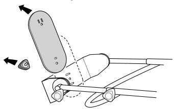
**1.** Remove the adjustment knob on the bottom of the foot plate. Remove the foot plate.
