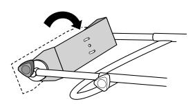
**3.** Rotate the foot plate bracket inward  $180^{\circ}$  as shown.
