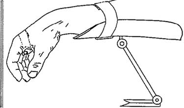
The joints also permit the forearm support to be tilted up or down. However, if this is done, the angle of tilt should be taken into account when setting the range of motion on the display.
