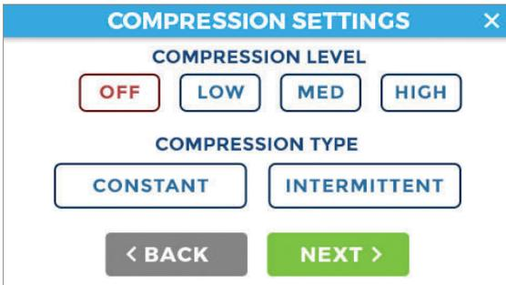
**STEP 4** Select desired COMPRESSION LEVEL and COMPRESSION TYPE and press NEXT.
