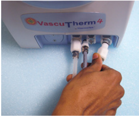
Disconnect umbilical from unit.
